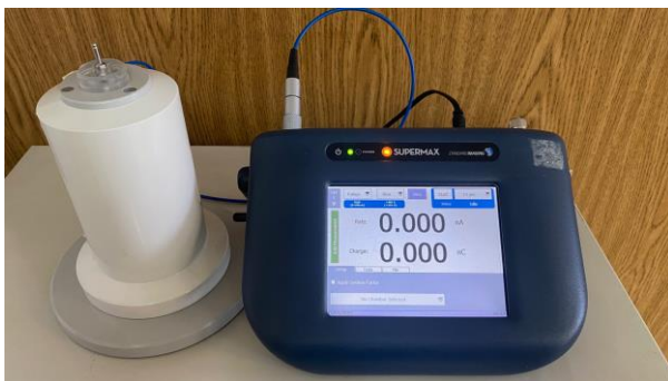
Dosimetry set (electrometer Supermax + well type chamber)
